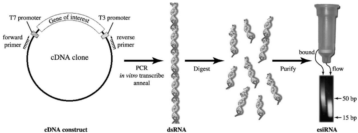
Fig. 1. Scheme for the preparation of endoribonuclease prepared siRNA. Important elements within the vector and the binding sites for the universal primers are depicted. An agarose gel from a typical esiRNA preparation is shown.
