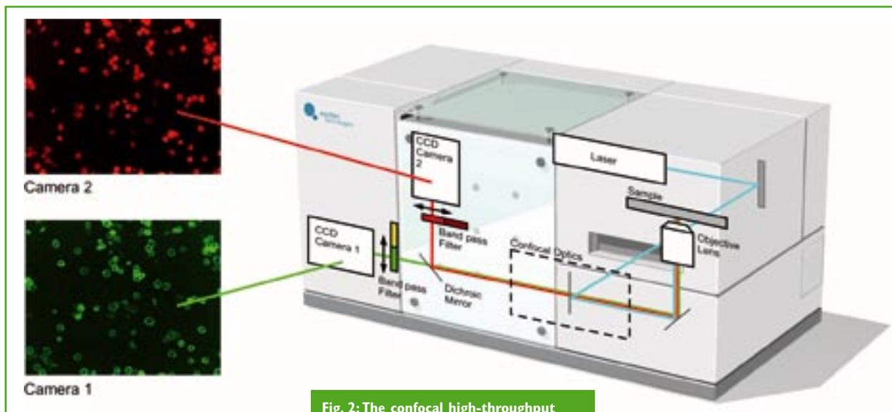
Fig. 2: The confocal high-throughput microscope Opera TEHS (Evotec Technologies GmbH, Hamburg)
