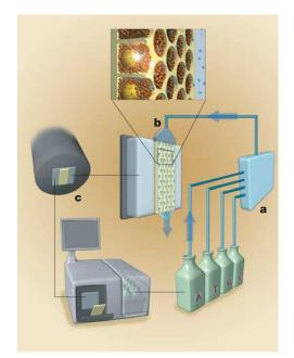
Figure 2 | Sequencing instrument. The sequencing instrument consists of the following major subsystems: a fluidic assembly (a), a flow chamber that includes the well-containing fibre-optic slide (b), a CCD camera-based imaging assembly (c), and a computer that provides the necessary user interface and instrument control.
