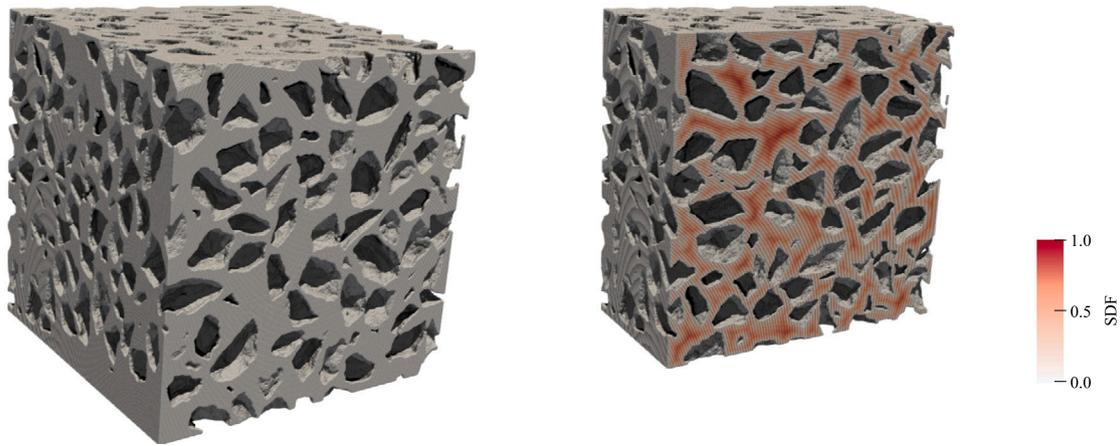
Fig. 5. 3D visualization of the sparse-grid level-set representation of the geometry from Fig. 4d. Left: full block; Right: clipped block with SDF values overlaid in color.
